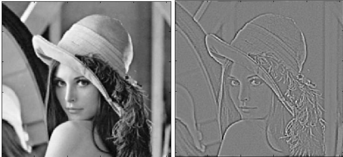
Figure 4: Original image and edge detected Image. In the analog VLSI image processor, the difference between two output images having different blur times performs edge detection.
